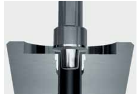
The front surface is continuously rolled and compressed. From the inside, the tube surface is slightly expanded to clamp the sleeve
