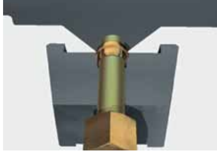
Tube is inserted into the tools until it firmly touches the stop at the end
