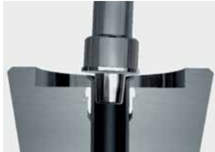
As soon as the flat working surface of the pin contacts the tube end, the flanging process begins
