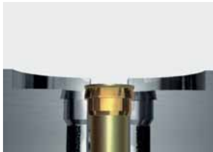
The tube end is released and can be taken out of the machine
